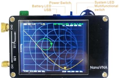
You can use the USB interface to connect to computer communications or connect standard 5V charger charging.
